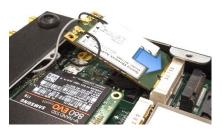
Insert the MODEM into the header. Ensure the antenna cables are not snagged or pinched and secure the MODEM using the silver bolt.
