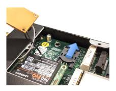
Lift the modem to the side to access the SIM holder. Slide the top of the SIM holder back to unlock it.
