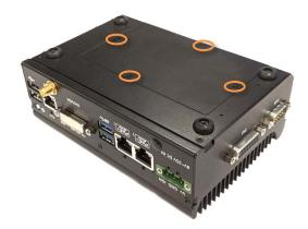
Unscrew and safely store the four black bolts holding the base hatch in place. Then remove the hatch.
