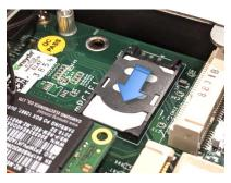
Close the SIM holder then slide it to lock the SIM in place.
