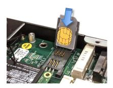
Lift the top of the SIM holder and insert the SIM card.
